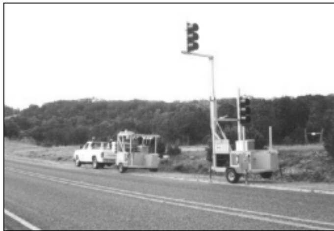
Figure 1. Field Setup of Portable Traffic Signals.
