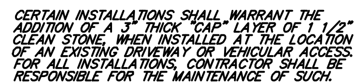
STABILIZED CONSTRUCTION ENTRANCE NOT TO SCALE
