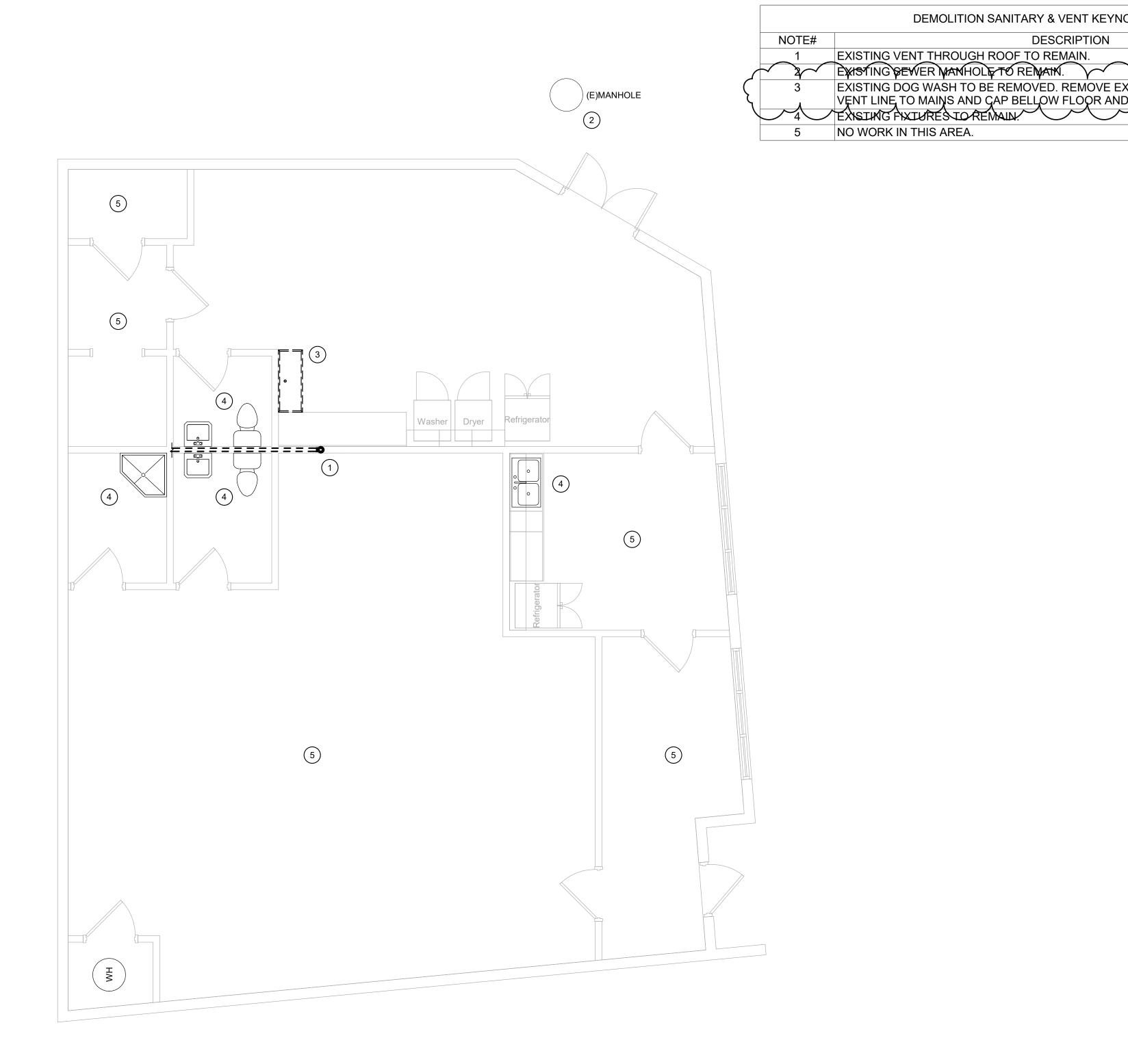
1 DEMOLITION SANITARY & VENT PLAN
