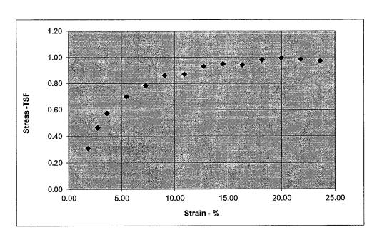
Unconfined Compressive Strength Failure Strain
